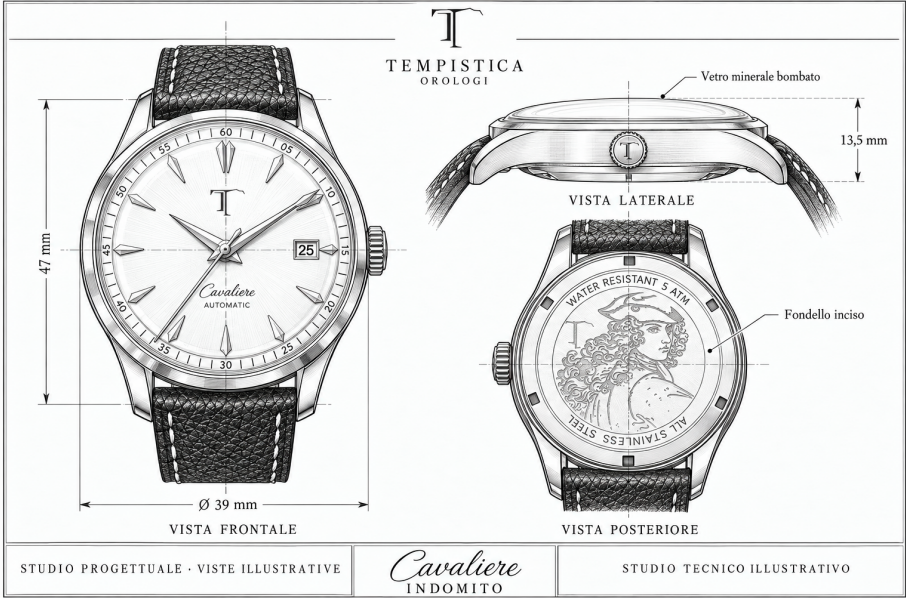
Front, side and rear views. Dimensions in mm.
